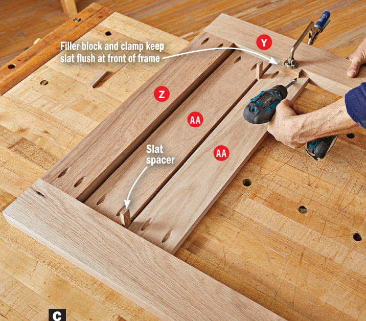
C Position the slats flush with the front of the frame as you assemble the doors. Spacers (about \frac{9}{32} " ) maintain equal gaps between the slats and the top and bottom rails.
