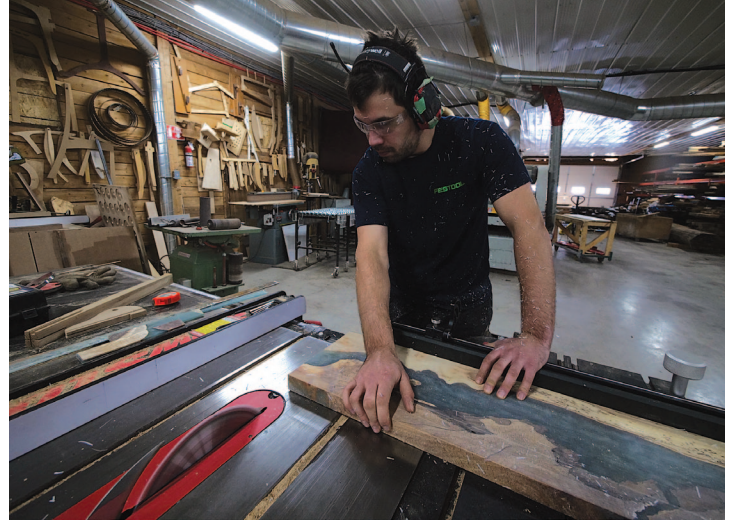
Machine Normally – Cured epoxy can be thickness planed and cut to size with a circular saw blade, like any regular piece of solid wood.
