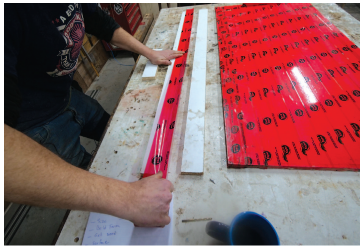
Cover it in Tape – Tuck Tape, a construction-grade adhesive tape, is applied to the inner surfaces of the form before the form is assembled. It will stop the epoxy from adhering to the form as it cures.
