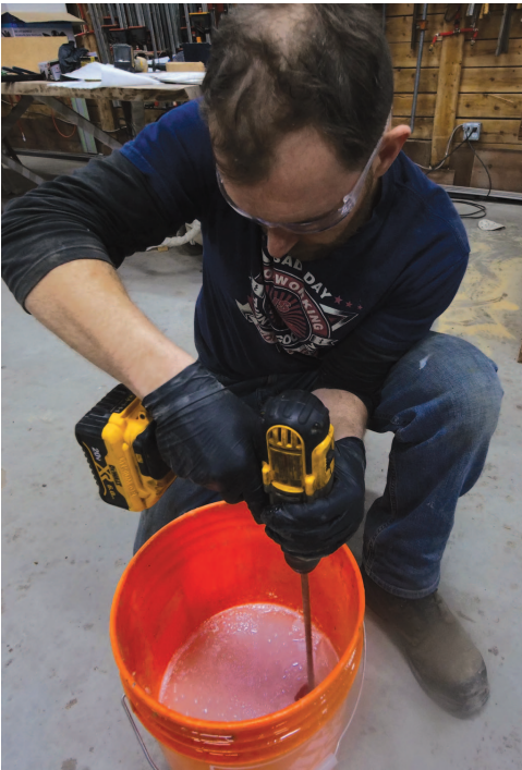
A Thorough Mix – A drill and a paint mixer does a good job of mixing up the epoxy. It's critical to ensure the epoxy is completely mixed or parts won't dry.
