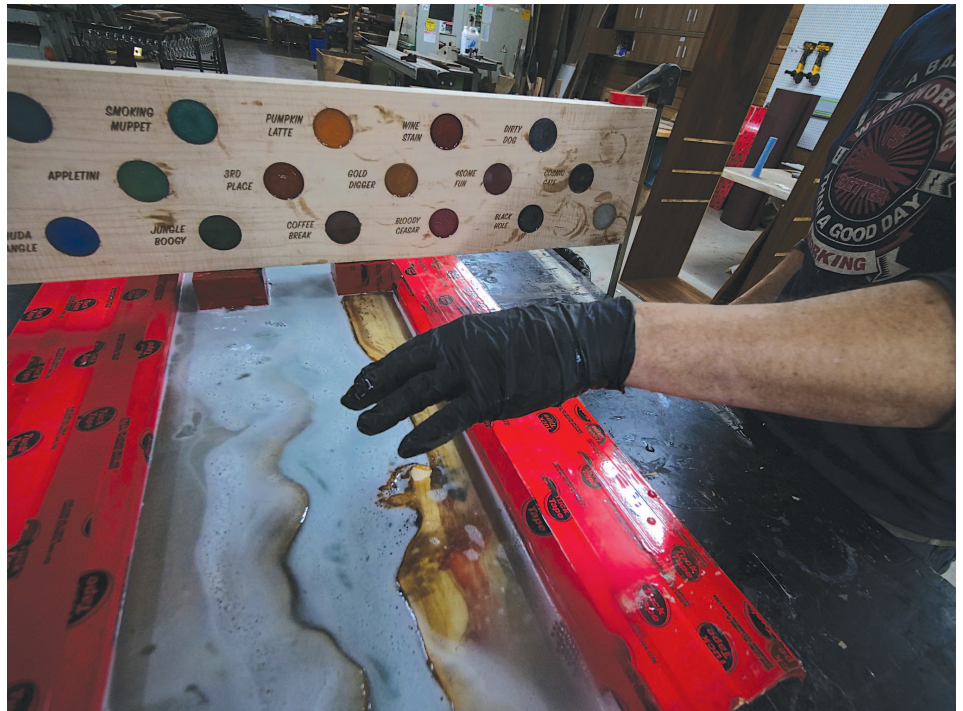
Flood the Form – Once mixed, pour the epoxy into the form and let it flow out. There's no reason to rush at this stage, as epoxy dries very slowly.
